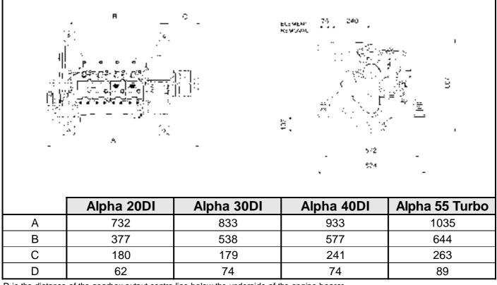
D is the distance of the gearbox output centre line below the underside of the engine bearer.
