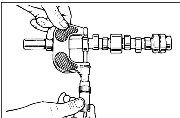
**CAMSHAFT LOBE MEASUREMENT PROCEDURE**
