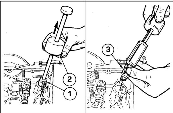
**PRE-COMBUSTION CHAMBER REMOVAL**
