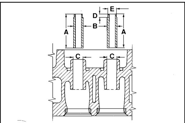
**VALVE GUIDES / VALVE GUIDE BORE**
