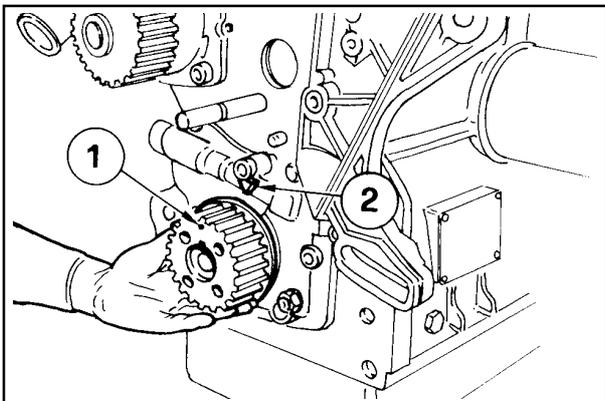
**CRANKSHAFT TIMING PULLEY**
