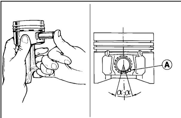
**PISTON WRIST PIN INSTALLATION / RETAINING SNAP RING**
