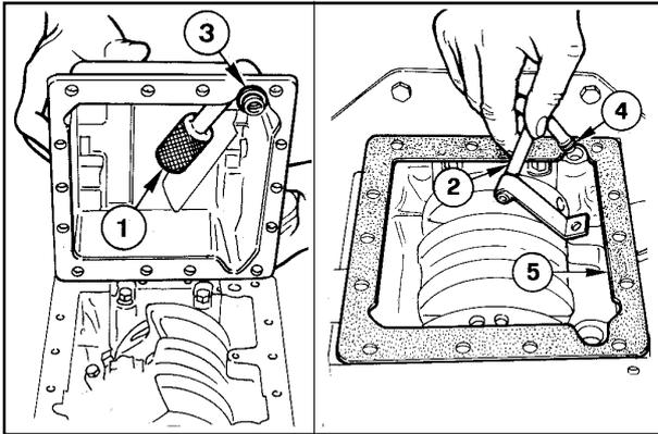
**OIL PICK-UP SCREEN AND OIL DRAIN BACK TUBE**
