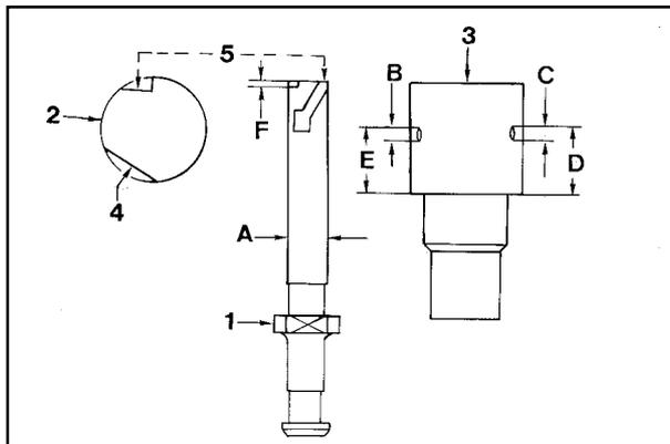
**BARREL AND PLUNGER DETAIL- (TYPICAL) CURRENT UNIT INJECTORS (EXAMPLE- 6590-285)**
