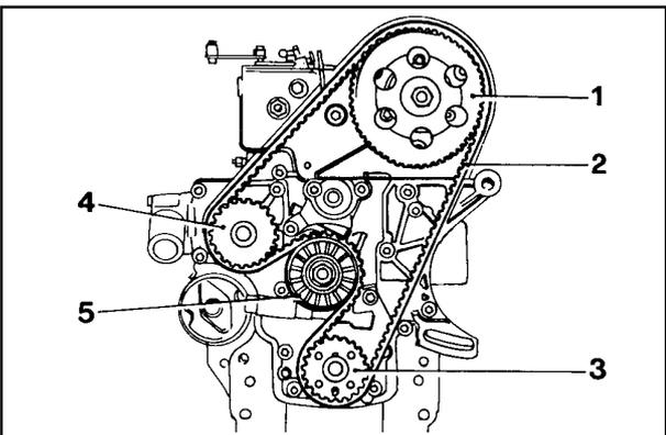
**TIMING BELT / TIMING PULLEY ARRANGEMENT**
