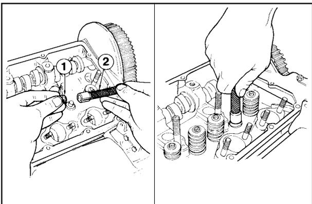
**VALVE STEM SEAL INSTALLATION**
