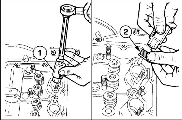
NOTE: THE PRE-COMBUSTION CHAMBER DOES NOT NORMALLY REQUIRE REMOVAL OR SERVICE AND SHOULD NOT BE DISTURBED UNLESS ABSOLUTELY NECESSARY. DO NOT REMOVE PRE-COMBUSTION CHAMBERS AS PART OF A NORMAL REBUILD OR VALVE JOB. FURTHER, LOMBARDINI RECOMMENDS THAT NEW PRE-COMBUSTION CHAMBERS BE INSTALLED IF REMOVAL OF THE EXISTING PRE-CHAMBERS IS REQUIRED. THE FOLLOWING PROCEDURES DETAIL PRE-CHAMBER REMOVAL AND INSTALLATION SHOULD SERVICE BE REQUIRED.
