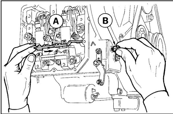
**INJECTION PUMP CONTROL ROD STROKE LIMIT ADJUSTMENT**
