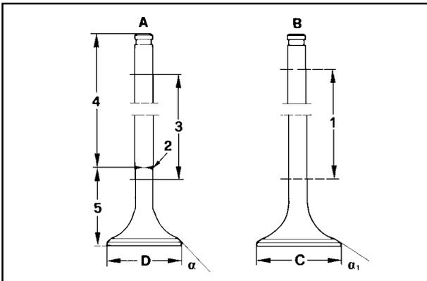
**INTAKE VALVE:** Base Material: X 45 Cr Si 8 UNI 3992
