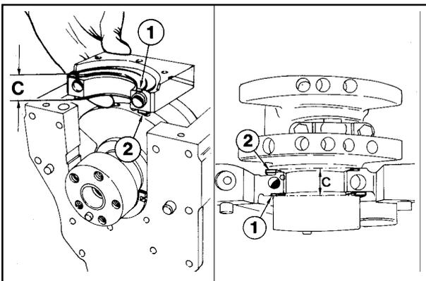
If the crankshaft end play exceeds the specifications above, fit the engine with oversize thrust bearing segments and/or grind the crankshaft thrust surfaces. The following provides guidelines for the application of oversize bearings and for grinding the crankshaft thrust surfaces.
