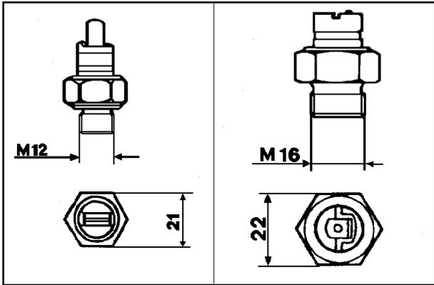
**OIL PRESSURE (LOW) SWITCH, COOLANT TEMPERATURE (HIGH) SWITCH**
