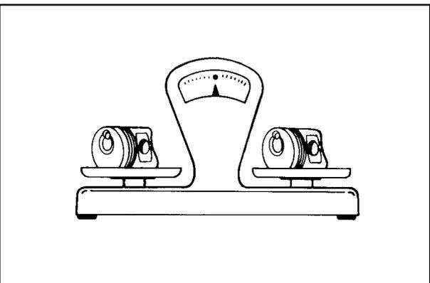
**REPLACEMENT PISTONS (SPARE PARTS):** Replacement pistons are supplied with piston rings reflective of the piston class. Replacement pistons are supplied as class A. Piston classes B and C are reserved for production engines. Oversized pistons are available as 0.50mm and 1.00mm and are supplied with piston rings reflective of the oversized diameter. DO NOT FIT PISTON RINGS FOR STANDARD PISTONS ON OVERSIZED PISTONS. DO NOT FIT RINGS FOR OVERSIZED PISTONS ON STANDARD PISTONS.
