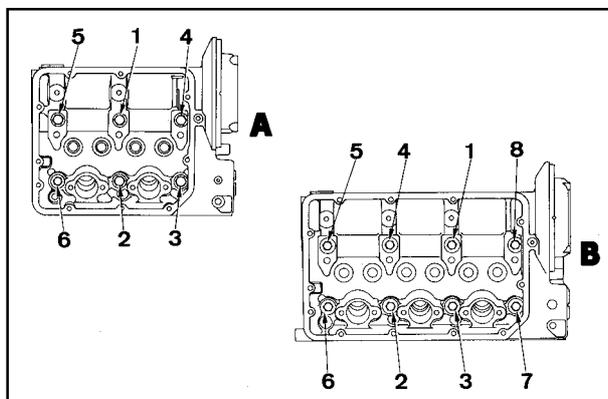
**CYLINDER HEAD TIGHTENING PROCEDURE- LDW 502, 602, 702, 903 and 1003:**
