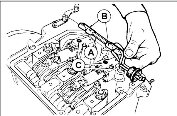
**UNIT INJECTOR CHECK VALVE**
