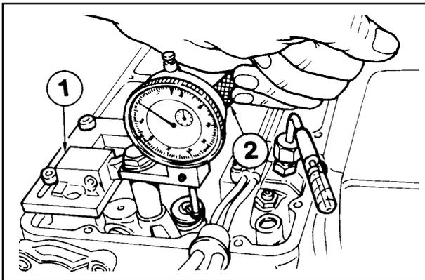
With the static injection timing instrumentation installed as described above, fit the engine with the timing fixture(1), part no. 1460-048 as shown. The dial indicator support should be oriented over the engine valve spring cap. Remove the injection pump rack assembly starting aid spring. Adjust and secure the injection pump rack at 1/2 stroke.
