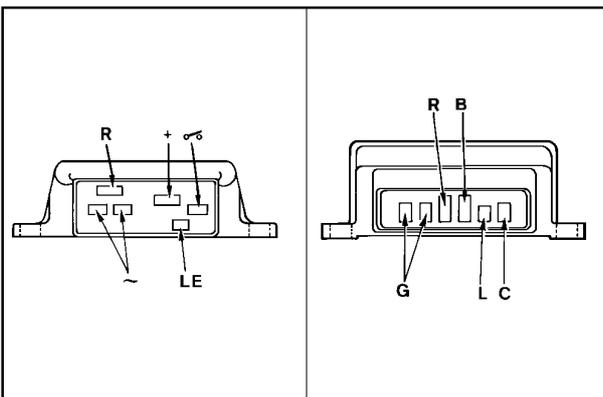
VOLTAGE REGULATOR CONNECTION DETAILS (FLYWHEEL ALTERNATOR ONLY)
