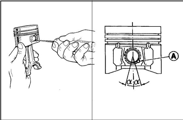
**PISTON / CONNECTING ROD DISASSEMBLY and PISTON INSPECTION**
