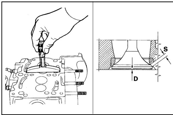
**VALVE RECESS and SEAT SEALING WIDTH**
