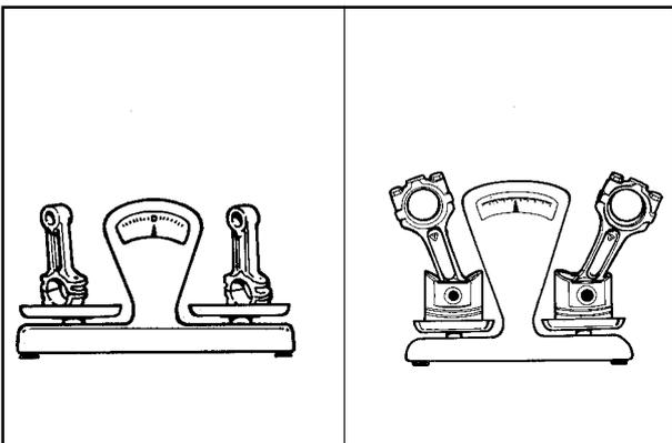
**CONNECTING ROD- PISTON ASSEMBLY BALANCE**
