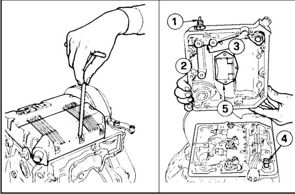
**VALVE / ROCKER COVER:** All critical engine adjustments require the removal of the valve/ rocker cover. Remove the valve / rocker cover by removing the crankcase vacuum regulator valve (see below), removing the retaining bolts, then lifting the valve / rocker cover assembly. The engine crankcase breather system is integrally contained by the valve / rocker cover. Additionally, the valve / rocker cover facilitates oil pressure measurement and camshaft/ rocker arm lubrication via oil ports.
