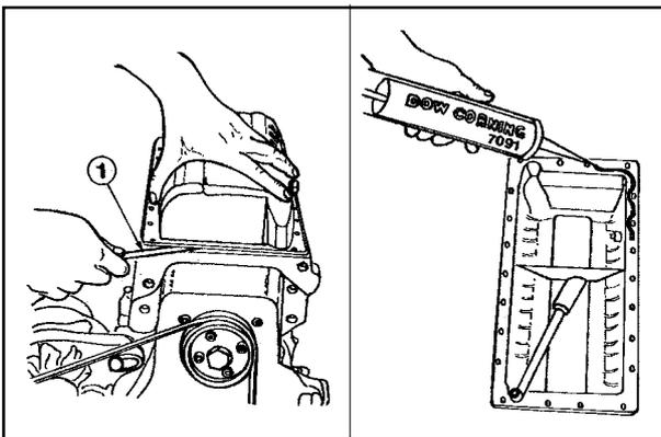
REMOVAL: Drain the oil from the oil pan. Remove all oil pan bolts. Gently, without deforming the pan, pry the pan from the crankcase using a small bar(1). Numerous attempts at several different locations around the perimeter of the pan may be required before the pan releases from the crankcase.
