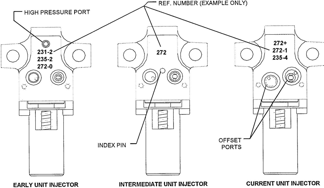
LOMBARDINI CONTINUALLY DEVELOPS THE FOCs DIESEL LINE. CONSTANT RESEARCH AND DEVELOPMENT IS CARRIED OUT TO IMPROVE OVERALL PERFORMANCE OF FOCs PRODUCTS. AS SUCH, THE DESIGN OF THE FOCs UNIT INJECTOR HAS CHANGED DURING THE DEVELOPMENT PROCESS. THE FIGURE ABOVE PROVIDES A REFERENCE FOR THE THREE(3) DIFFERENT VERSIONS OF THE FOCs UNIT INJECTOR TO DATE.
