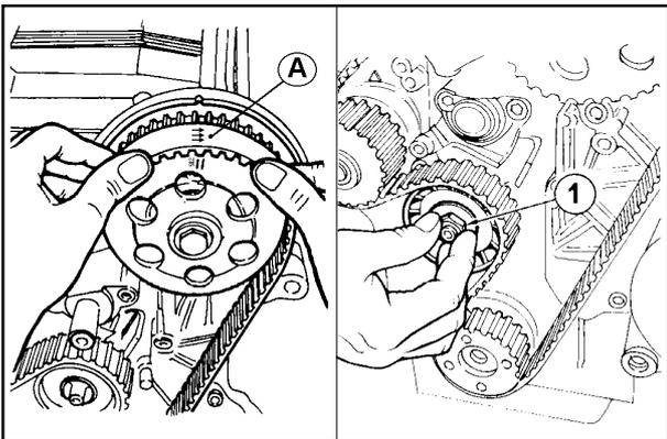
**TIMING BELT INSTALLATION- TIMING PROCEDURE**
