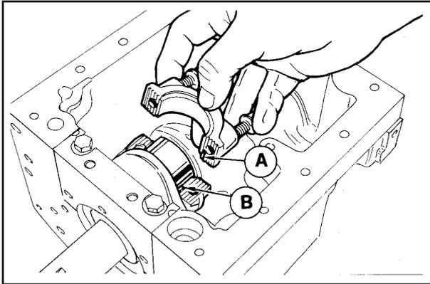
**CONNECTING BEARING / ROD CAP INSTALLATION**
