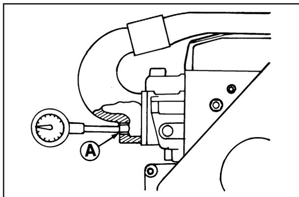
**TURBOCHARGER PRESSURE TESTING**
