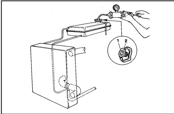
**COOLING SYSTEM PRESSURE CHECK / RADIATOR CAP INSPECTION**
