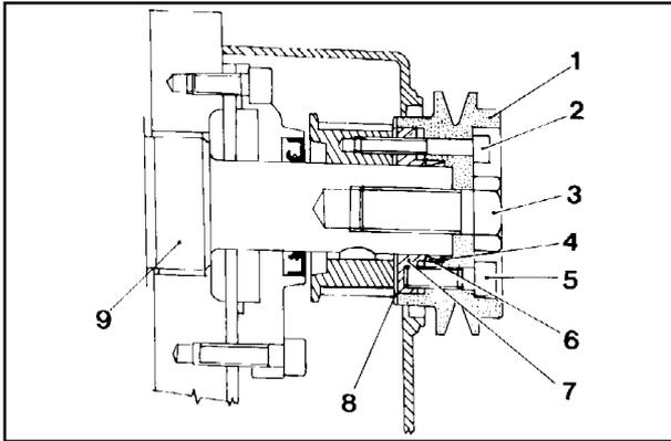
**No. 2 PTO (CRANKSHAFT PULLEY) with "RINGFEDER"- LDW 1204, LDW 1204/T, LDW 1404**
