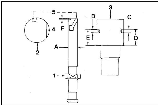
**BARREL AND PLUNGER DETAIL- EARLY UNIT INJECTORS (TYPICAL)**
