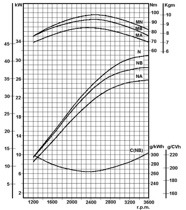
**N** - 80/1269/CEE- ISO 1585, Gross automotive rating- intermittent operation with variable speed and variable load.
