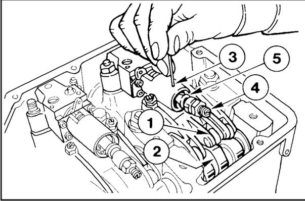
**UNIT INJECTOR REMOVAL / INSTALLATION**
