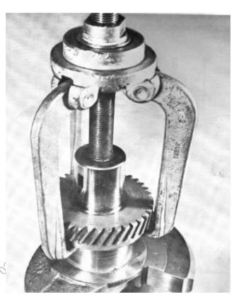
**36.** Place the key in the crankshaft's key slot. Heat the gearwheel to approximately 100°C (212°F) (no more) and press it onto the crankshaft. Note! The marking on the gearwheel shall face outwards. Refit the circlip on the crankshaft.
