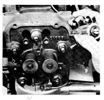
**78.** Lubricate and replace the valve lifters. Fit a new cylinder head gasket and then the cylinder head. Place the washers under the nuts and tighten the nuts in three stages to 70 Nm (7 kpm) (50Lbft.). See the tightening sequence.
