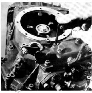
6. Fit tool 884078 to the flywheel. Afterwards screw in the centre screw on the tool until the flywheel loosens.
