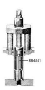
**46.** New valve guides are fitted with tool 884549. Use a press. This tool gives the guide the right height above the cylinder head's valve spring seat surface. Check the dimension "A" - this must be 9 mm (0,3543 in.) when the guide is pressed into place.
