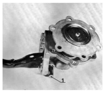
32. Remove screw 1 and withdraw the manual pump arm 2 and replace spring 3 if it is broken. Note! Be careful of the rubber seal which is pressed into the housing.
