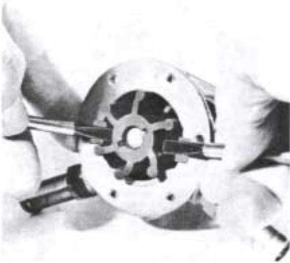
46. Unscrew the bolt and pull the impeller off the shaft. If the sealing rings also have to be replaced, the shaft can be pulled out entirely together with the impeller, after which the bolt can be released.
