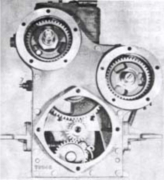
63. Place a new gasket on the water pump and fit it with the two bolts. Make sure that the groove in the pump shaft engages in the flange nut.
