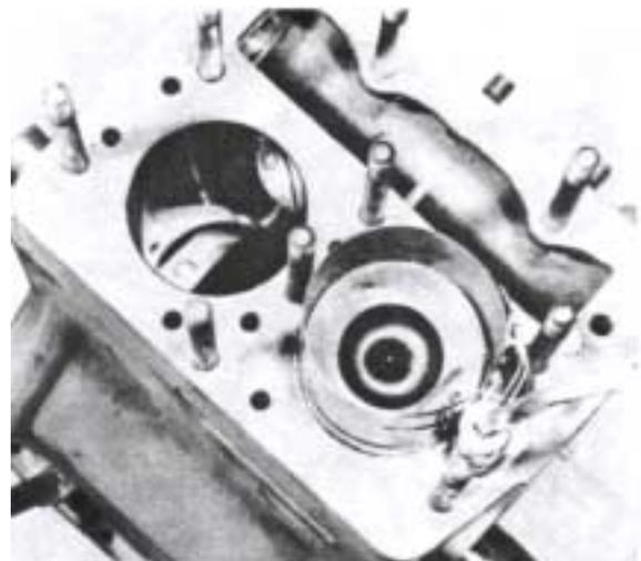
53. Fit the "protective cover" for the starting crank. Replace the sealing ring and gasket.
