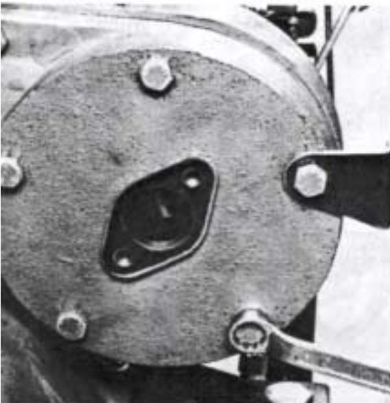
64. Fit the cover with new gasket over the camshaft end. NOTE! The bolts have three different lengths. The Fig. below shows where they are placed.
