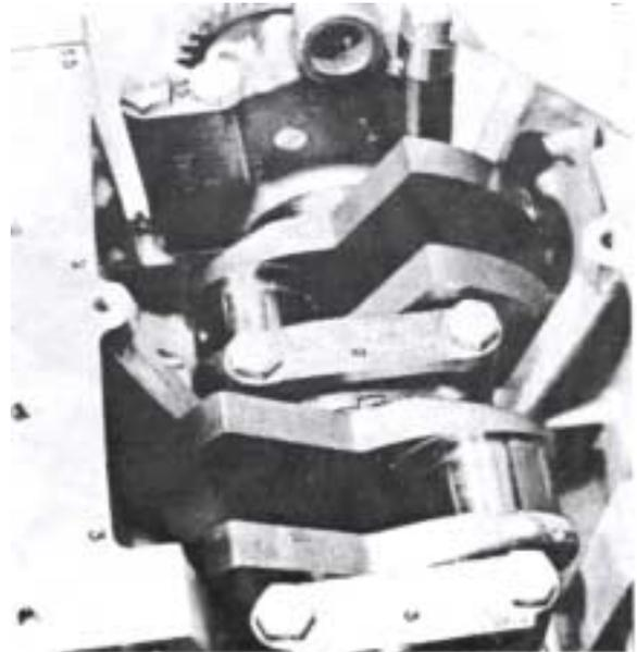
52. Turn the piston rings so that their respective gaps are apart from each other. The piston top is marked with "Front" and should point towards the flywheel. NOTE! Fit the connecting rod which is marked with punch pops nearest the flywheel. Carefully tap the piston downwards through the installation tool with a wooden handle or similar. Place the engine on its side and tighten up the caps. Tightening torque = 50 Nm (5 kpm = 36 lbfft). Lock the bolts with the lock washers.
