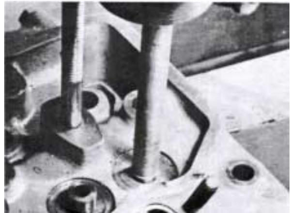
30. Remove the seals on the valve stems. Remove the valve springs with the help of a valve spring remover. Remove all the collets 1. Remove the valves. IMPORTANT! Place the valves in the order in which they are removed. Discard burnt valves if the wear is excessive and grind valve seats if necessary (See under Technical Data). Seats and valves must be ground together so that the contact surfaces will be absolutely tight.
