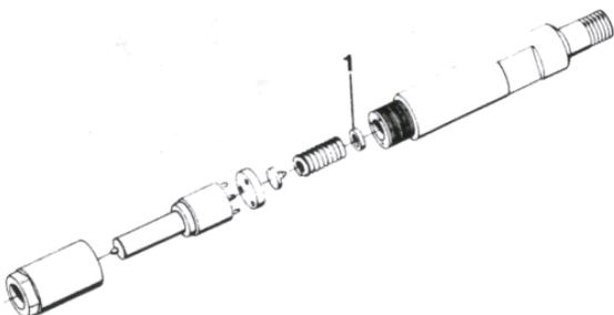
40. Release the cover centre screw, lift out the strainer 1 and clean it.
