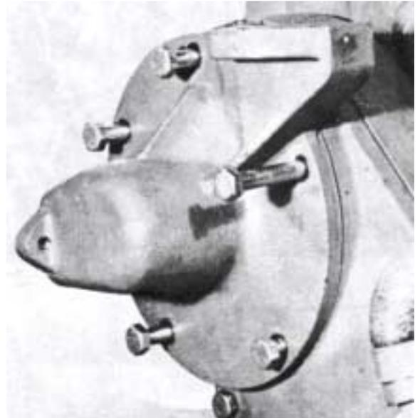
65. Install the fuel pump. Make sure that the 0-ring is in position. Use a new 0-ring. The pump is installed with two inhex bolts and spring washers. Check that the pump "squeaks" by pressing in the pump lever before installing the pump on the engine. Connect up the fuel hoses.
