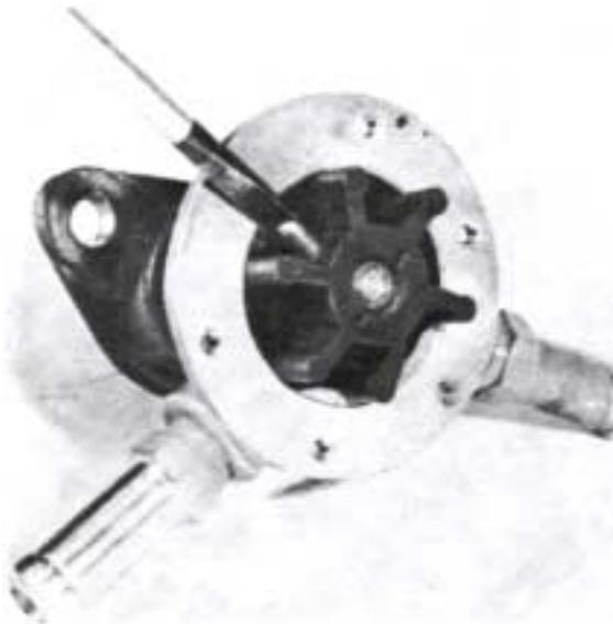
47. Remove the sealing rings 2 and the 0-ring 1 (earlier engines), and clean the pump body and shaft. (**IMPORTANT!** The pump must be removed from the engine.) Check to make sure there is no burr on the shaft. **NOTE!** A new 0-ring must not be fitted.
