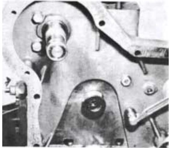
54. Fit the camshaft. Observe due care so that the sealing ring in the protective cover for the starting crank is not damaged. Knock the starting crank pin into the camshaft. Use a tube or similar as a counterhold.
