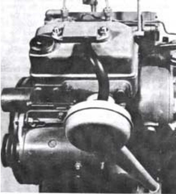
79. Fit the key in the crankshaft. Heat the flange and fit it on the shaft. Tighten it up with the bolt and the thick washer. Tightening torque: 80 Nm (8 kpm = 57 lbfft). Bend down the thin washer over the bolt head. Fit the rubber damper.
