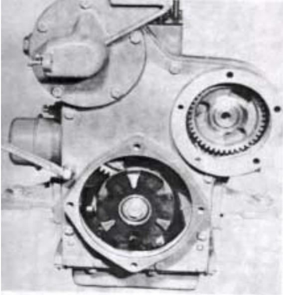
11. Knock out the hand starter pin in the camshaft. Remove the protective cover (2 bolts). NOTE! Scrap the sealing ring and fit a new one.
