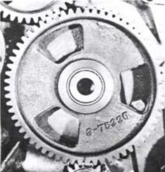
59. Install the fuel injection pump. Use a new gasket. Fit the key on the pump shaft and install the gear wheel. **IMPORTANT!** The figure must face towards the figure on the intermediate gear. Tighten up the gear wheel with the nut which also functions as a flange for the water pump. Tightening torque = 60 Nm (6 kpm = 43 lbfft). Use a counterhold. Tighten the camshaft nut. Remove the counterhold.
