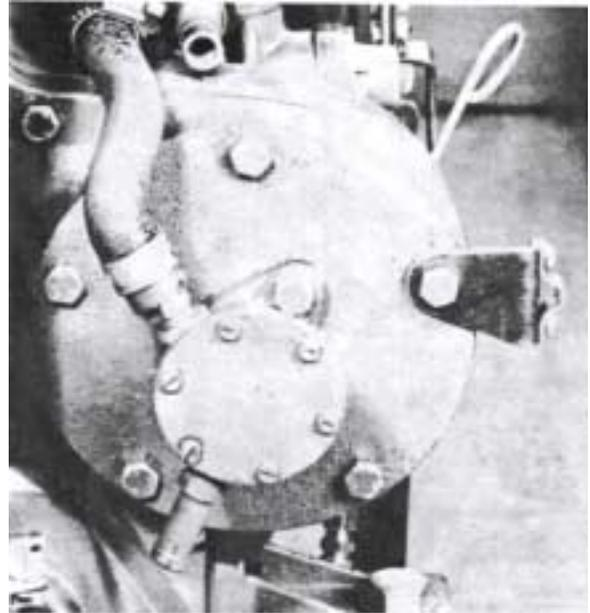
62. Fit a new gasket and cover where the water pump is to be installed. NOTE! The control bracket is fitted with one of the bolts. Two bolts are shorter.
