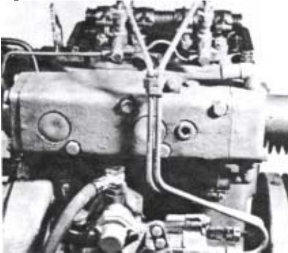
75. **Adjusting the BOSCH injection pump**
