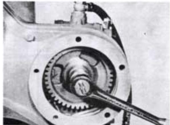
9. Remove the timing gear cover. NOTE! The small round cover on which the fuel pump is mounted has bolts with 3 different lengths. The bolts for the large casing has two lengths. The bolts for the large casing has two lengths. The two bottom bolts are shorter than the others. Carefully lever loose the timing gear casing from its guide pins. Discard the gasket.
