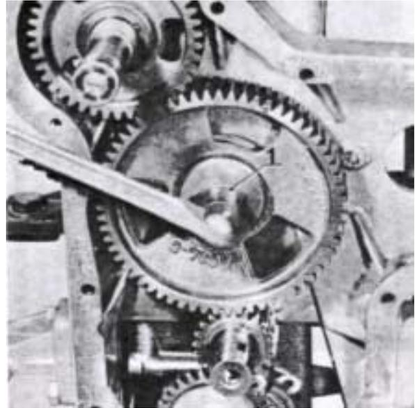
14. Bend down the lock washer and release the bolt securing the reverse gear flange to the crankshaft. Use a counterhold. NOTE! Take care of the key. Lever loose the rubber damper with a screwdriver.
