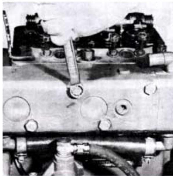
5. Remove the rocker arm cover (2 nuts), the intake manifold (4 bolts), the rocker arm (2 nuts) and the cylinder head (9 bolts). Take care of the washers.
