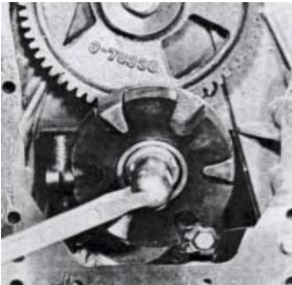
16. Check that the shaft pin 1 for the intermediate gear is secure.
