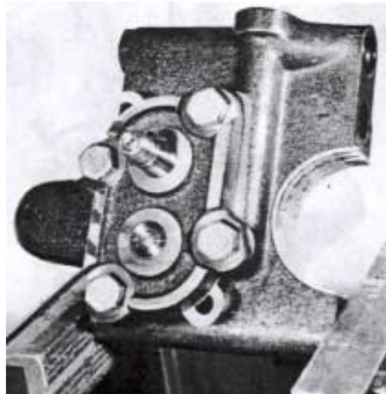
25. Re-fit the gears as shown in the Fig. below. Fit the cover together with a new gasket. Tighten up the 4 bolts and rotate the shaft to make sure that it does not jam. Fit the key in its groove and re-fit the gear wheel. Fit the spring washer and tighten up the gear with the nut.
