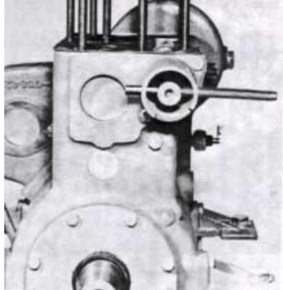
10. Remove the flywheel. Remove the nut and use a puller. The axle is tapered and provided with a key. Use a counterhold when releasing the nut.
