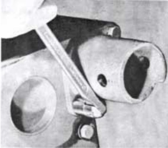
55. Fit a new gasket and install the timing gear casing (4 bolts). Tap carefully so as not to deform the guide pins.
