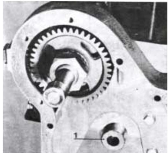
57. Fit the intermediate gear. Check that the punched-in figures on the crankshaft drive and camshaft gear wheel coincide with the marking on the intermediate gear.
