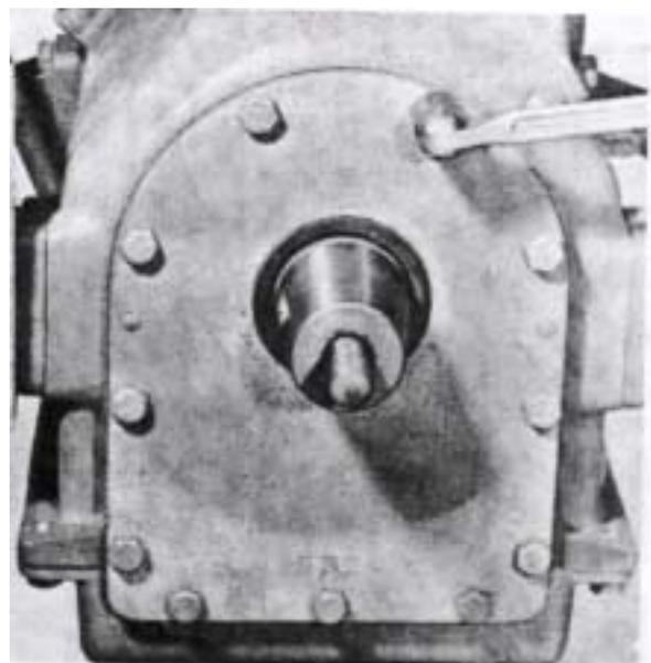
13. Remove the sump as well as the nut and lock washer for the camshaft. Use a counterhold on the crankshaft.
