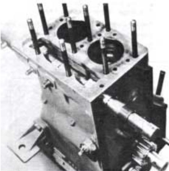
56. Fit the key in the camshaft and then the gear wheel. Turn the gear wheel so that the figure which is punched on the ring gear faces outwards. Fit the star washer and the nut on the camshaft. Tighten up later on (see Point 59). When a new engine block is used, a new shaft pin 1 for the intermediate gear must be fitted.
