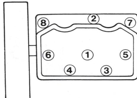
61. Place a new gasket on the inner timing gear cover and fit the outer timing gear casing. Two short bolts are fitted at the bottom. Trim off any part of the gasket which sticks out.
