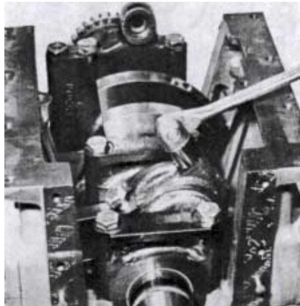
21. Mark the connecting rod and cap nearest the fly-wheel with a peener. Peen as shown in Fig. 21.
