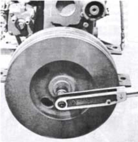
71. **MD6A.** Install the stars generator with its bracket. Screw tight the tensioning bar to the engine. Earlier engines have a washer placed between the engine and bracket.
