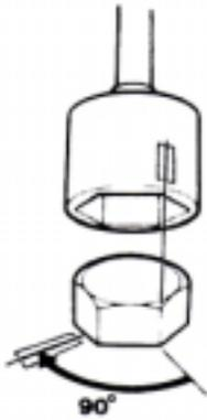
Tightening using both a torque setting and a protractor angle requires that first the recommended torque is applied using a torque wrench and then the recommended angle is added according to the protractor scale. Example: a 9Q0 protractor tightening means that the joint is tightened a further 1/4 turn in one operation after the stated tightening torque has been applied.
