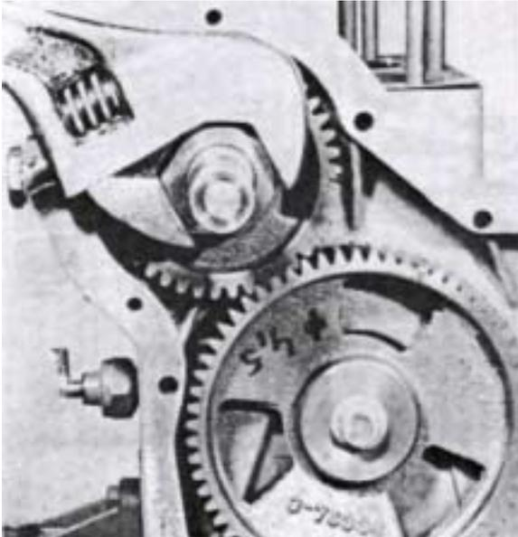
15. Remove the bolt for the intermediate gear. Discard the sealing washer 1 under the bolt. Pull off the intermediate gear.
