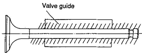
Apply lubricating oil down to the lower surface (hatched portion in the figure) of the valve guide before reassembling the valve stem.
