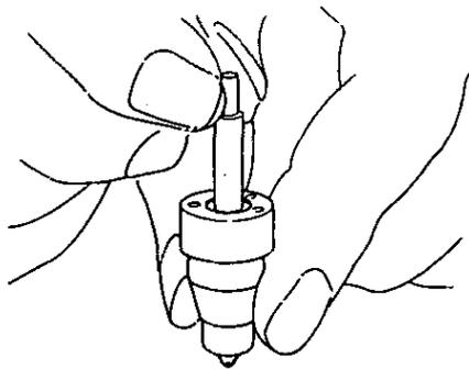
( Nozzle valve sliding check by gravity )
