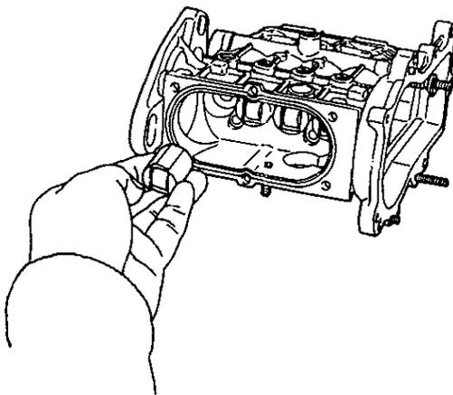
(14) Take out the plunger, plunger spring and plunger spring lower retainer from the lower part of the fuel injection pump.
