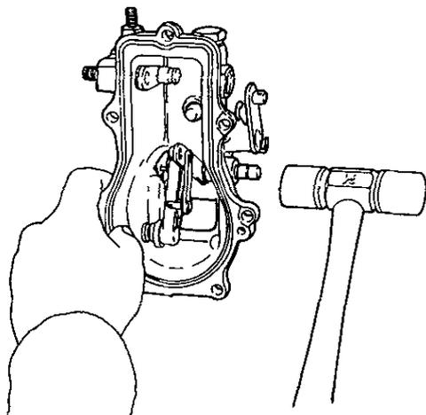
\* After mounting the governor lever assembly, make sure the governor lever assembly moves smoothly.
