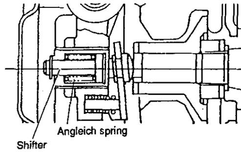
**6. Inspection of torque spring assembly**
