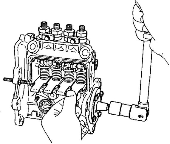
(16) Fix the fuel injection pump. Using a mallet, tap the end of the fuel injection pump camshaft to adjust the side clearance of the fuel injection pump camshaft using an adjusting packing and a side clearance gauge (special service tool).
