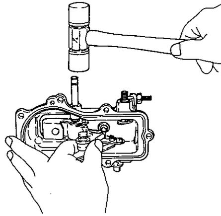
\*2. Make sure to insert the governor lever shaft in the correct direction.
