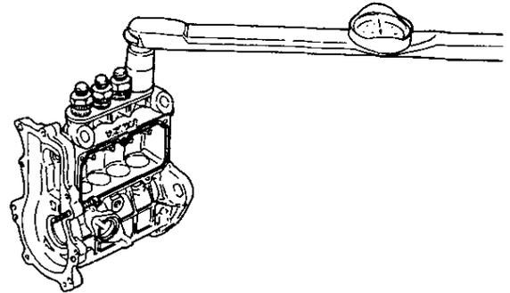
(20) Tighten the holder stopper to the specified torque.
