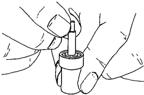
( Nozzle valve sliding check by gravity )
