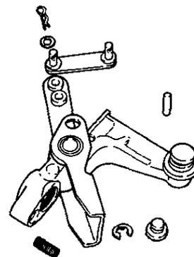
\* The governor assembly consists of the governor lever, tension lever and angleich, and is normally not disassembled.
