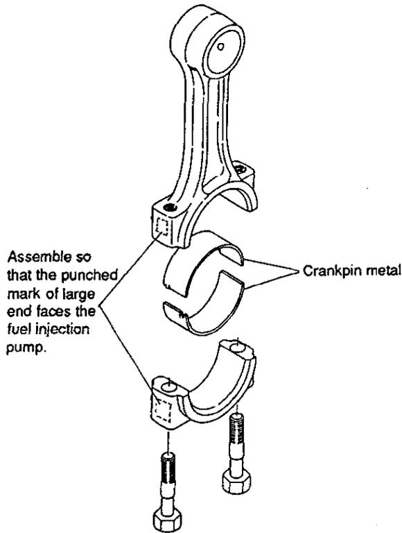
**6. Assembling the piston and connecting rod**
