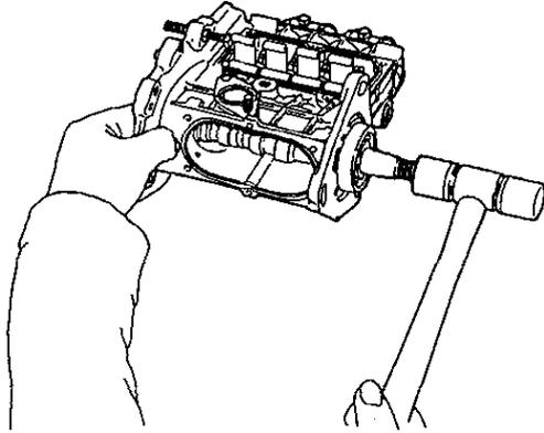
(13) Fit the oil seal to the inner side of the bearing holder. Mount the bearing holder.
