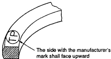
2. Assemble the piston rings to the cylinder, staggering the piston rings joints at 120° intervals, making sure that they are not aligned along the piston. Apply lube oil to the circumference of the piston.
