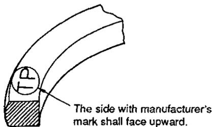
(2) Stagger the piston rings joints at 120° intervals, making sure that they are not aligned along the piston. Apply lube oil to the circumference of the piston.
