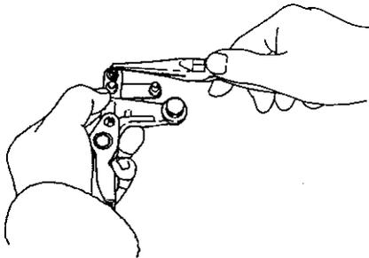
(7) Put the governor lever shaft assembly in the governor case, insert the governor lever shaft and tap it in until the O-ring groove comes out the opposite side of the governor case. (for DI)
