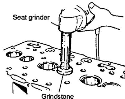
**[Procedure for Using The Seat Grinder and Seat Cutter]**
