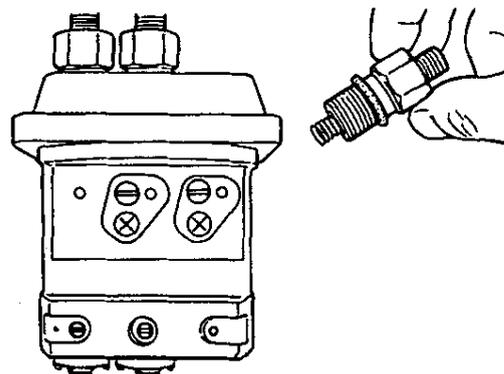
(7) Remove the plunger barrel assembly.
