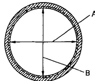
Note: Measurement should be made at a, b and c in the directions of A and B.
