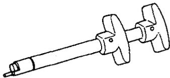
( Special service tool: Plunger insertion tool )
