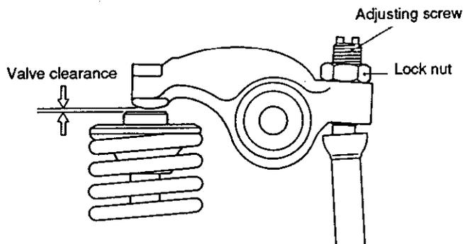
(Adjusting the valve head clearance)
