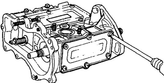
(19) Tighten the delivery valve spring holder to the specified torque.
