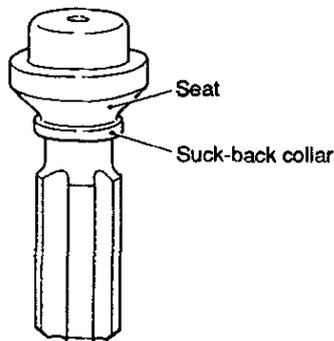
2. Stop up the hole in the bottom of the delivery valve holder and keep the seat as it is. Insert the delivery valve to the holder. While releasing your upper finger, check to see if the delivery valve springs back. If so, it is acceptable.
