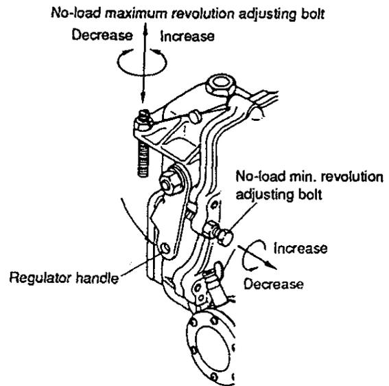
\* : The illustration shows the partial perspective view of the governor for the direct injection system.
