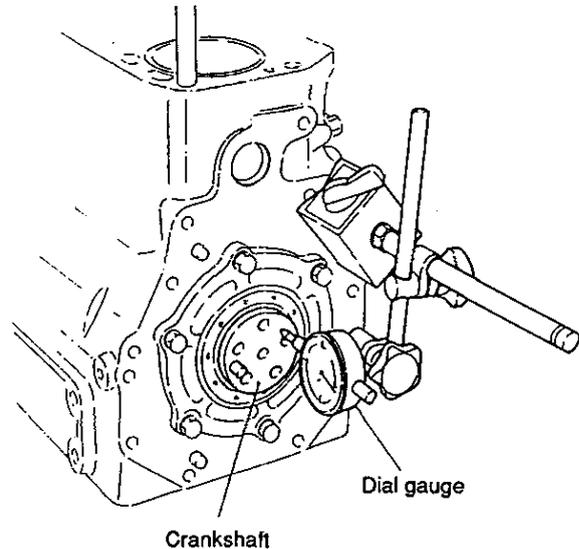
( Measurement of side gap around )
