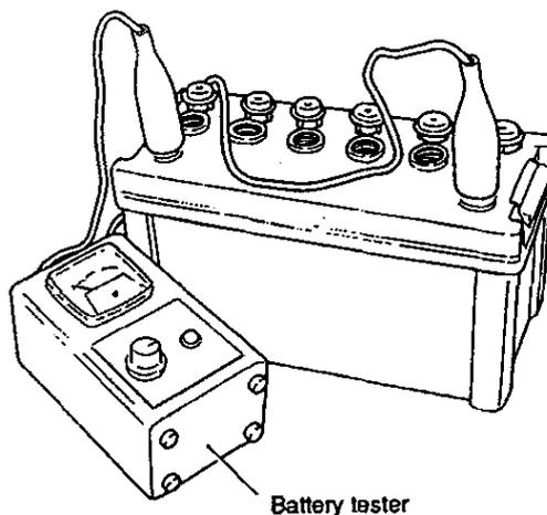
( Measuring the battery charge with battery tester )
