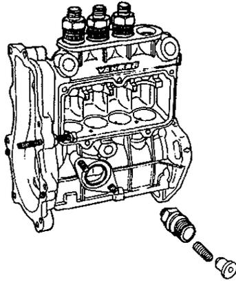
(20) Take out the plunger barrel toward the upper part of the fuel injection pump.
