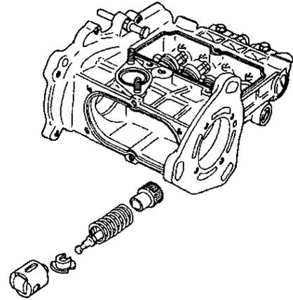
(15) Remove the stop screw from the fuel control pinion.
