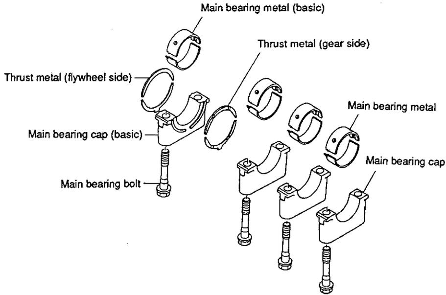
**7. Undersized main metal by 0.25 mm and the oversized thrust metal by 0.25 mm**
