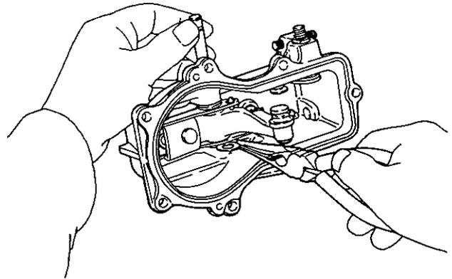
\*3. Don't forget to mount the washers on both sides of the governor lever.
