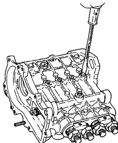
(12) By using the handle of a hammer, etc., push up the plunger guide from the bottom of the pump and take out the tappet holders (special service tool).
