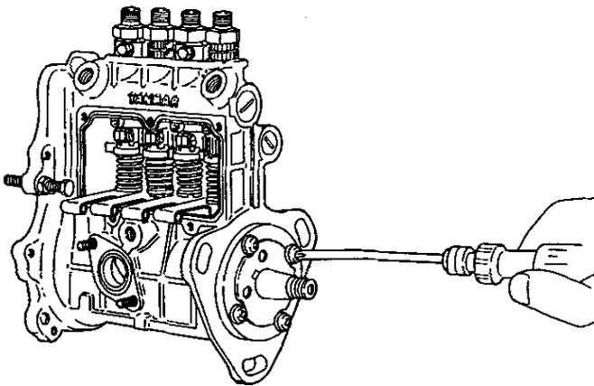
(14) Drive the woodruff key into the fuel injection pump camshaft.
