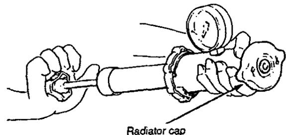
(Checking the radiator cap)
