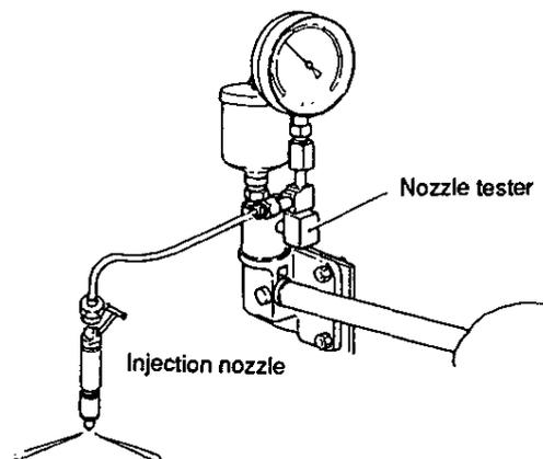
( Measuring the injection pressure with )
